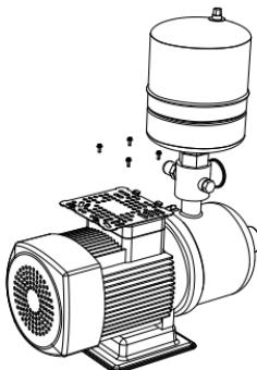
**Step 3:Install the bottom plate**
