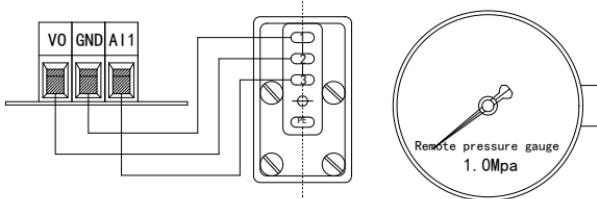
(2) **Pressure transmitter**: working voltage range 10 ~ 30V, output 4 ~ 20mA. Wiring method is shown as below.
