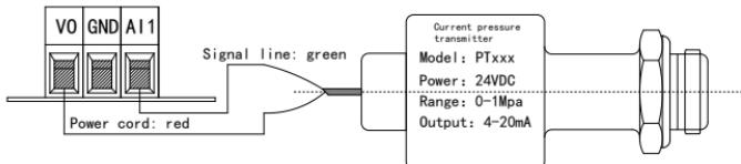
Notes: Model for PDM30-2SXXX products will be equipped with dedicated sensors (red line connected to terminal +VO; black line connected to terminal AI). For the wiring method of various sensors and the setting of relevant parameters, please refer to appendix.
