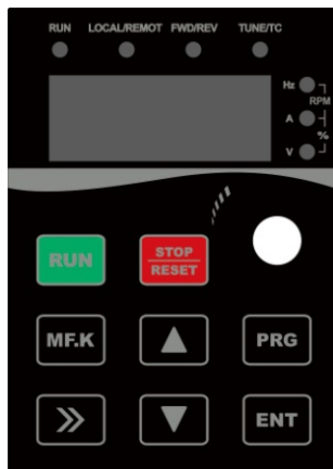
Figure 4-1-1 Keypad Schematic Diagram
