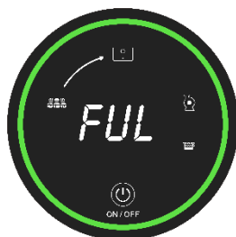
Tank Full State (Tank Full Indicator On)
