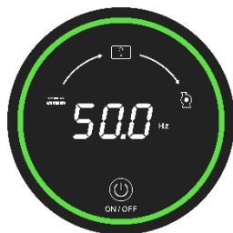
DC Input Running Mode (Green Light Ring Rotates)
