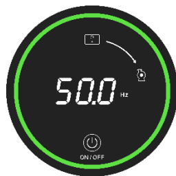
AC Input Running Mode (Solar Array Disconnected)
